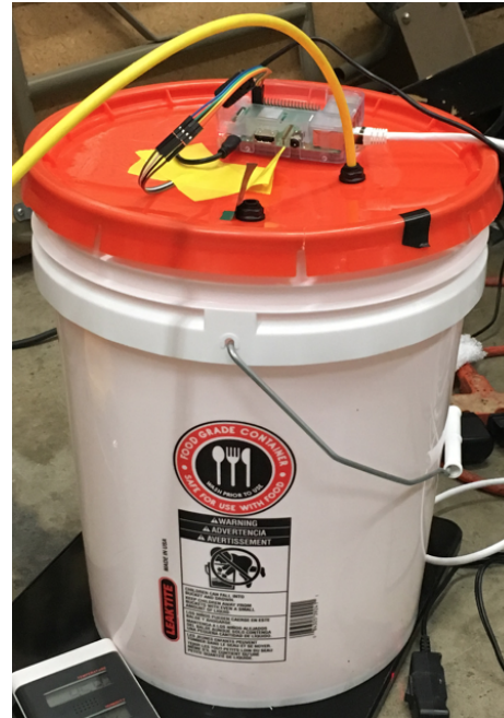
Fig. 4.10: View of the testing bucket with attached electronics.
