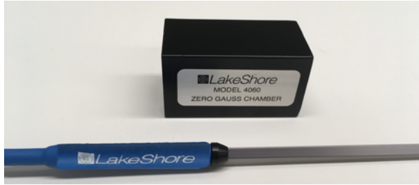
Fig. 3.13: Lakeshore hall probe and zero gauss chamber for calibration.
