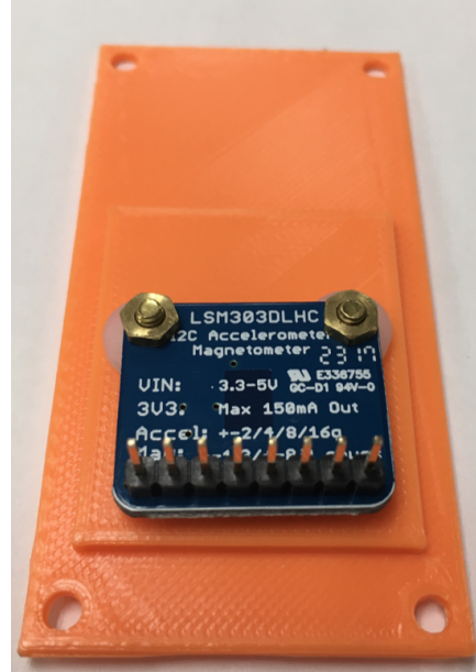
Fig. 3.12: Photo of the lid with a magnetometer attached.
