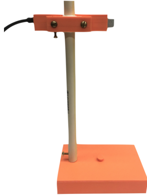
Fig. 3.14: Metrolab hall probe in custom 3D printed stand for calibration.
